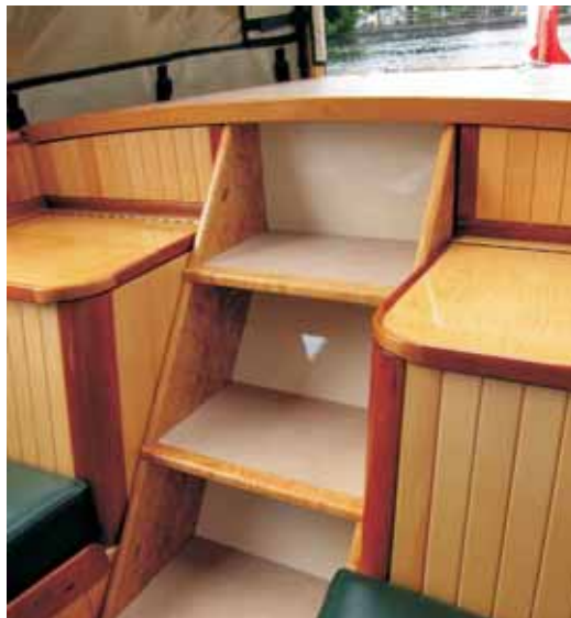
Left—The white cedar paneling either side of the aft stairs is trimmed with cherry.
