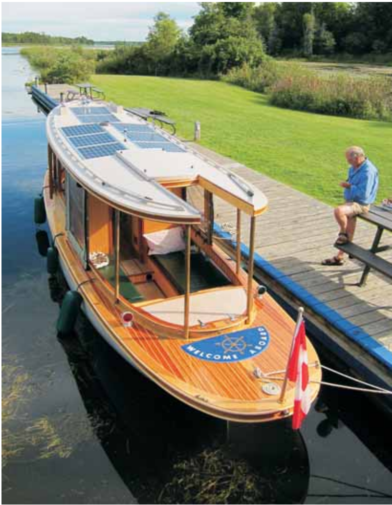
Ted Moores relaxes after tying up Sparks for the night at Kilmarnock Lock. While there is daylight, the solar panels will continue to charge the batteries for another day's travel on the Rideau Canal.
